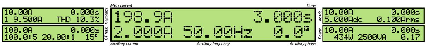
The 200ADM-P Mk2 has a flexible auxiliary AC output that can be used at up to 260V for voltage relays or up to 10A for current relays. The phase and frequency of this output are fully adjustable. This combination of voltage and current allows testing of relays that require two voltages, one voltage and one current or two currents.
