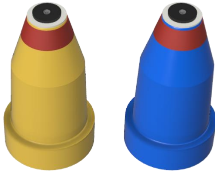
Figure 2 The Comparator Transmitter (TX—Yellow Cone) and the Comparator Receiver (RX—Blue Cone)
